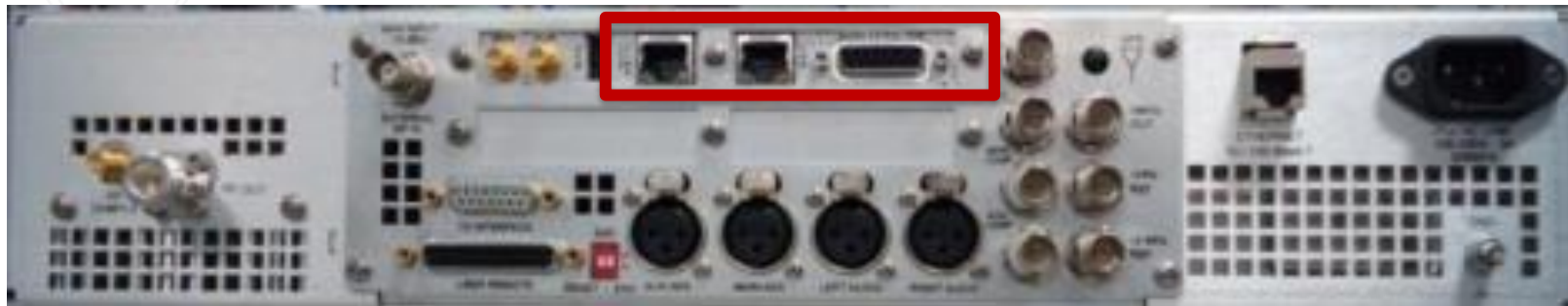
GatesAir Dig. Modulator Card Installed in Flexiva FM Exciter
